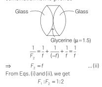
**53** Two identical glass ( $\mu_a = 3/2$ ) equi-convex lenses of focal length f each are kept in contact. The space between the two lenses is
